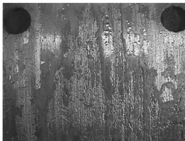
Fig. 2 Features on the contact surface of the brake shoe. Shiny areas are retained patches of friction films. Some areas show blisters. The distance between the rivet holes is 57 mm (optical image).
